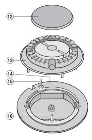
Be careful not to mix up the parts. Make sure that all the locating tabs and notches align exactly.
